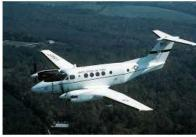
Wingspan: 55 ft Length: 44 ft Height: 15 ft Color: White Rate of Climb: 2,500 ft/min Approach Speed: 115-130 KIAS
