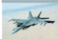
Wingspan: 44 ft Length: 60 ft Height: 16 ft Color: Grey Rate of Climb: 6,000+ ft/min Approach Speed: 130-150 KIAS
